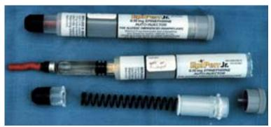
Intact (upper picture) and dismantled EpiPen (lower picture) to show the spring, needle and syringe that is enclosed within the EpiPen device.
